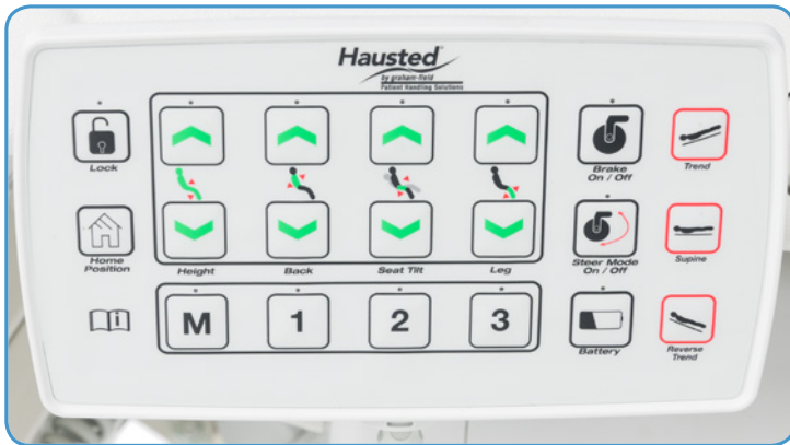
POSITIONING AT YOUR FINGERTIPS: Intuitive Hand Pendant with Pre-Sets and 3 Memory Positions
